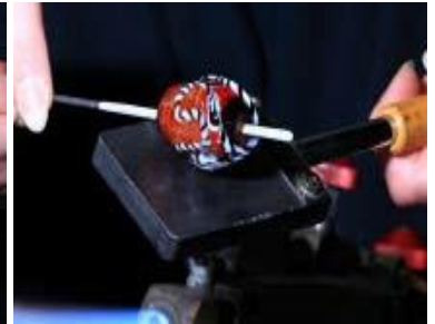
16. Final bead shaping then get the bead hot and molten.
