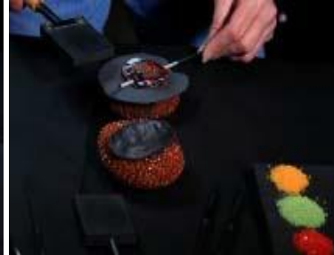
19. Quickly remove graphite paddles used to press glass or it will chill the glass.
