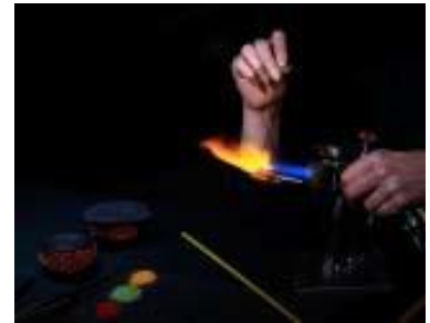
5. Build up molten glass around mandrel that has been dipped in bead release.
