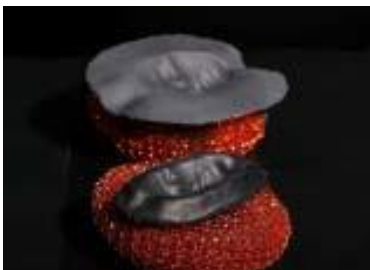
4. Molds sprayed with dry graphite and placed on copper scrub pads to cushion the mold while pressing molten glass into it.
