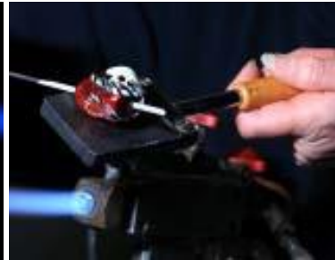
15. Shaping bead with graphite paddle.
