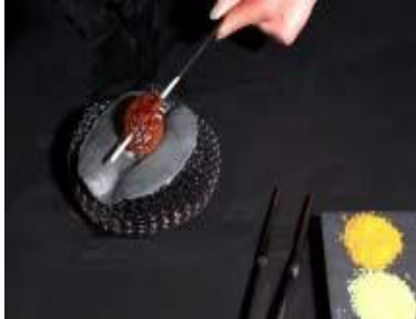
17. Quickly lay bead into mold supported with copper scrub pad.
