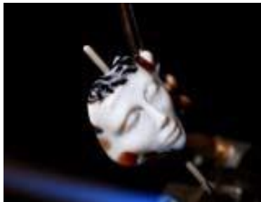
22. Place finished bead into annealing.
