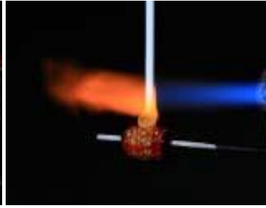
11. Adding volume for face to frit into mold.
