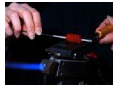
8. Shaping molten glass bead.
