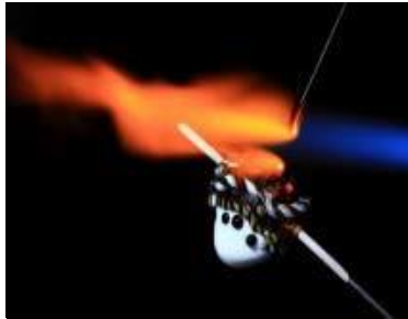
14. Using flame to cut glass from rod.
