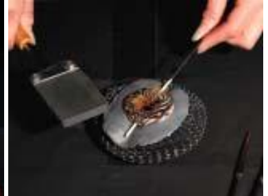
20. Give a light tap to the mold and pull the bead out of the mold.
