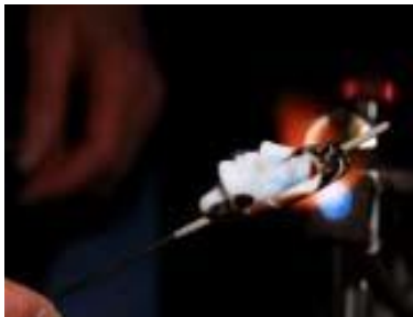
21. Fire-polish any chill marks caused by graphite paddle. Keep face out of flame. MM6 does not cause chilling, so there is no need to fire-polish the face.
