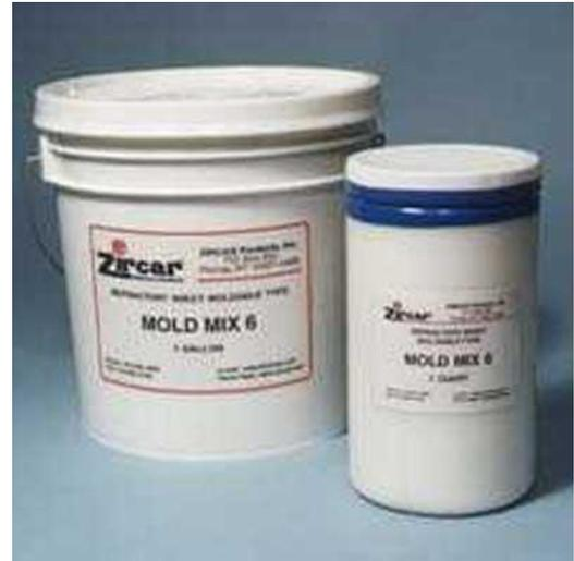
Mold Mix 6 is composed of high strength alumina fibers and alumina powders. Mold Mix 6 is ideal for use up 1550°C (2822°F) and above. It will air dry within 48 hours at room temperature or can be force dried with heat. When dried and fired to temperatures above 300°C (572°F), it is extremely strong and resilient.
